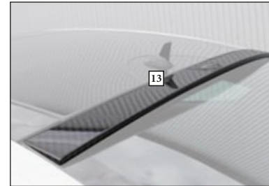
13. Roof spoiler ..... C204 630 841 visible carbon fibre primed without clear coat
