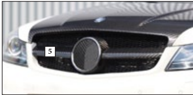
5. Front grill mask visible carbon fibre primed without clear coat
