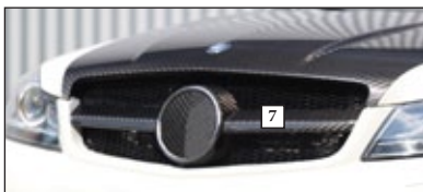
7. Front grill mask visible carbon fibre primed without clear coat
